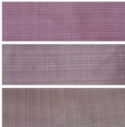
Figure 7: The dyed silk cocoon fabric after one wash, two washes, and three washes, respectively, showing a gradual change to a lighter shade and lesser intensity compared to the original color
